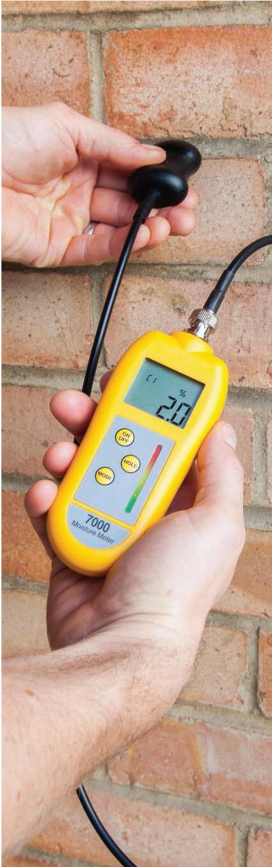
We manufacture a range of portable, pin-type (resistance) moisture meters for both the professional and the craftsman. Pin-type moisture meters are acknowledged as a reliable way to obtain percentage moisture readings in a wide range of building materials. The relationship between moisture content and electrical resistance provides consistent and accurate results over the range of 4 % to the fibre saturation point, which is approximately 30 %, dependant on the material.
