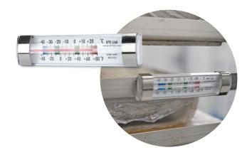
This spirit-filled fridge/freezer thermometer is encased in a clear ABS housing ( $20 \times 30 \times 122$  mm). The thermometer's colour-coded zones indicate temperature over the range of -40 to 20 °C and -40 to 80 °F with a 1 °C resolution.
