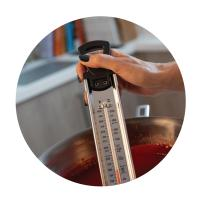
This stainless steel thermometer indicates temperature over the range of 40 to 200 °C and 100 to 400 °F in 2 °C/°F divisions. The thermometer's stainless steel casing incorporates a retaining clip and measures 50 x 240 mm plus a 65 mm plastic handle.
