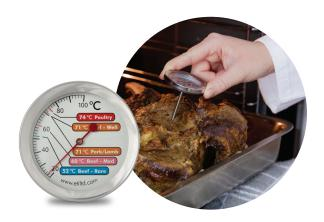
This meat dial thermometer features a large Ø60 mm dial with a Ø5 x 102 mm stainless steel pointed probe. The unit indicates temperature over the range of 20 to 100 °C in 2 °C divisions.
