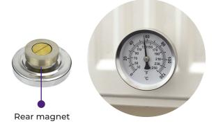
This Ø60 mm stainless steel, surface dial thermometer incorporates a magnetic sensing pad for mounting on ferrous metals and indicates temperature ranges from 0 to 120 °C or 32 to 250 °F.
