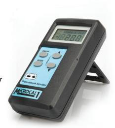
Thermocouple type K Range -200 to 1372 °C Thermocouple type J Range -200 to 1200 °C Thermocouple type T Range -270 to 400 °C Thermocouple type R Range 0 to 1768 °C Thermocouple type N Range -200 to 1300 °C Thermocouple type S Range 0 to 1768 °C Thermocouple type E Range -140 to 1000 °C
