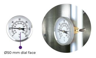
This easy-to-use surface pipe thermometer indicates temperature over the range of 0 to 120 °C or 32 to 250 °F. The Ø50 mm dial face has a clear, graduated scale indicating temperature in 2 °C and 4 °F divisions. Ideal for use in hot water pipework.
