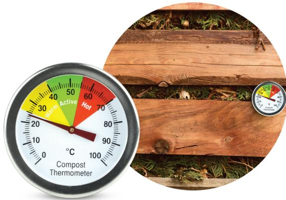
This bi-metal dial compost thermometer incorporates a colour-coded, easy to read dial. A compost thermometer is an important piece of equipment for any good gardener, in respect of ascertaining the temperature of any compost heap.
